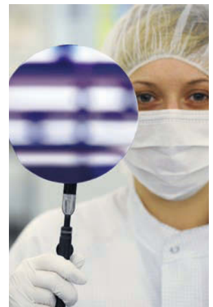
Osram Opto Semiconductors is in the pilot stage of producing high-performance blue LEDs that it grows in GaN layers on 6-in. silicon wafers rather than the current, more expensive sapphire wafers.
